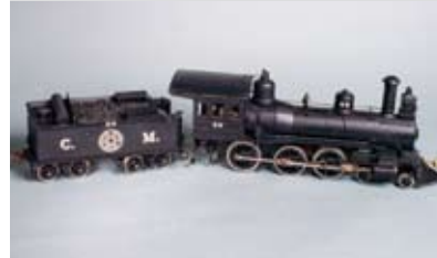
MEW #105 4-6-0 "Colorado Midland" Steam Engine & 4 Freight Cars (7/16" Scale) 1965 Designed and imported from Japan by Dick Wheeler. Modeled on the Colorado Midland #25, Class 93, built by Schenectady Locomotive Works in 1887. A modified version of this engine was used for distant shots of the Hooterville Cannonball featured frequently in the 1960s sitcom "Petticoat Junction."
